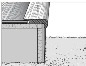
1. Beginning at the riser, measure and cut a piece of laminate to fit flush with the subfloor.
